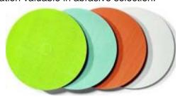
Trizact film, which consists of precisely shaped pyramids containing micron graded abrasive material bonded to specific backing. As the Trizact product is used, the tops of the pyramids wear away, continually exposing fresh abrasive material. This ensures a consistent cut rate during the life of the product.
