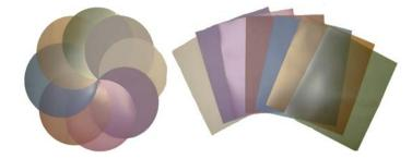
PSI Diamond Lapping Film is available in 4 specifications and 11 micron grades with or without a Pressure Sensitive Adhesive (PSA) backing. All share a precision 3 mil polyester backing, color coded for easy grade identification. The types differ in the method used to secure the diamonds particles to the polyester film backing.
