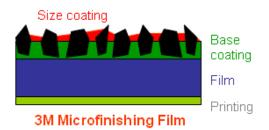
Product flatness is achieved and maintained through the grinding steps by the consistent 5 mil caliper of the dense, polyester backing. Unlike the traditional paper products, the abrasive particles cannot "recede" into the backing. This feature results in shorter grind times and longer life because the abrasive particles remain at the "cutting" interface. Shorter grind times mean less heat generation in the material ground. Longer life means improved economics.
